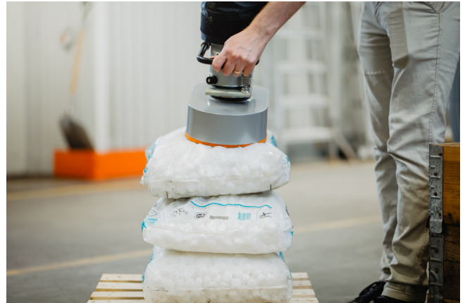
A bag lifter spares the back — Lifting heavy bags and sacks with a bent or twisted back results in an increased risk of musculoskeletal disorders. Lifting devices are often a good solution to avoid musculoskeletal disorders among the personnel when the work cannot be reorganised or automated.
