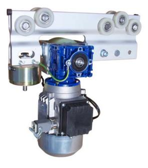
Powerdrive is an electric drive unit for Mechrail, integrated in the rail system trolleys. The driving speed is stepless, adjusted by frequency converter and controlled by a joystick.
