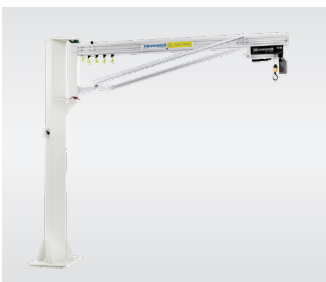
Under-braced jib crane arm
